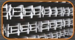
■ Common grades: As per IS 2062 : 2011 ■ Dimensional Tolerance: As per IS 808 : 1999
